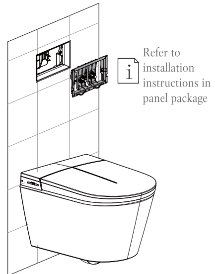
22 Install flush control panel
